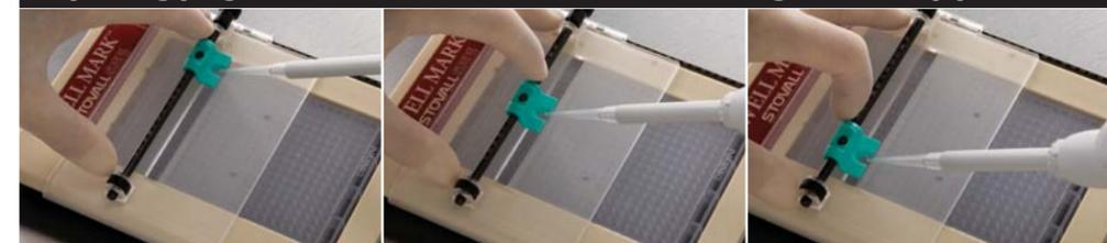
A similar set of detents on the shorter index bar provides the same alignment for the single-well isolator as the operator moves it down the column from well to well.
