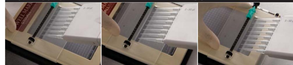
The protective, slotted cover is moved by the operator from one column of wells to the next while the other hand dispenses reagent from a multi channel pipette. The protective slotted cover shields adjacent columns of wells from accidental contamination and registers the current dispensing position.
